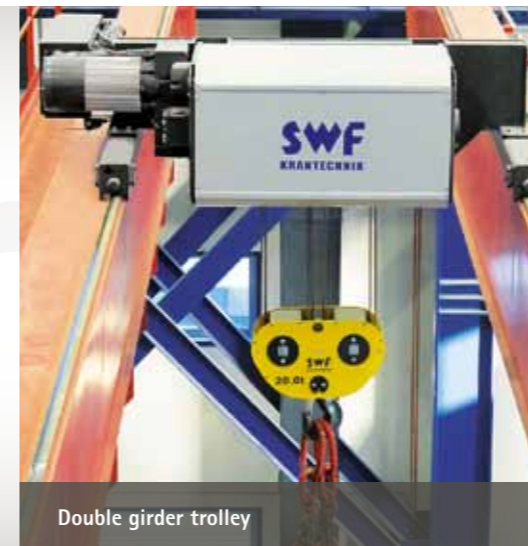
S-motor with encoder and external fan
