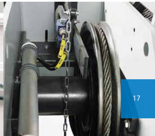
State-of-the-art electrics Gentle inclination Trolley travelling motor with PLIOTEX type wire marking Central lubrication Free accessible pulleys and hook operated ultimate hoisting limit switch
